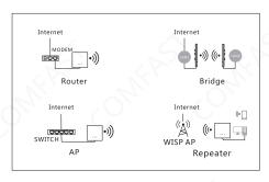
6. Click AP mode and set up IP Address and Subnet Mask. The IP address and Subnet mask should be within the same network segment as upper network and can't be conflict with IP address from upper network router. After settings, you can visit the device from the IP address you have set just now by connecting internet with WAN port of the device or POE adaper LAN port.
